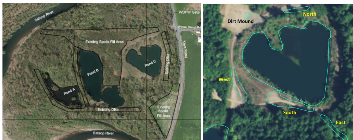
Figure 1. Satsop Ponds Pre-Restoration Footprint (left). Lines approximate positions of ponds, dikes, and spoils areas. Temporary (Auxiliary) Ponds (right) associated with permanent Pond C at the Satsop Restoration Sites
